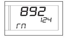
show the total number of hours that the treadmill has been operated. An "E" for English miles or an "M" for metric kilometers will appear in the lower left corner of the display. Press the Speed + button to change the unit of measurement if desired.
